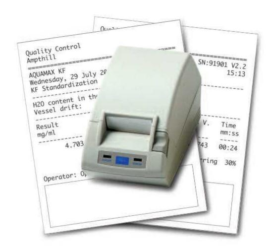
Following data will be printed (or sent to PC) after a titration or standardisation: Header, date and time, reagent factor, drift value, sample ID code, titration result, final volume, titration duration, user name.
